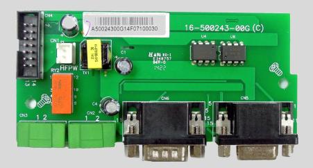
This accessory is applicable to select 48VDC models of HS and MS series inverters. It is a required component to be installed in every unit of a parallel system. A parallel kit includes:
