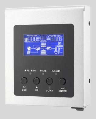
This device is an extension of the HS/MS inverter's LCD module and allows user to implement control on settings and monitoring from a distance away, one unit at a time.
