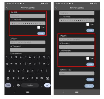
Step 8: After entering the value of the baud rate, click the "Save" button to complete the setting of Uart Baud Rate.
