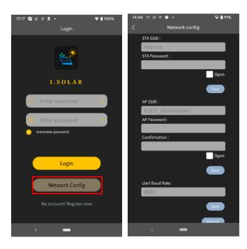
Step 4: After the Wi-Fi connection is successful, click the i.Solar App installed on the phone to enter the login page. Then, click the "Network Config" button to enter the Wi-Fi configuration page.
