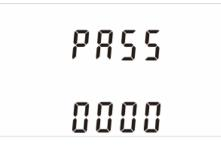
Setting up is password-protected so you must enter the correct password (default '1000') before processing.
